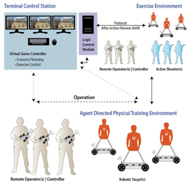
*The TCS Provides Shared Virtual Environment for Operator and Scenario Control*
